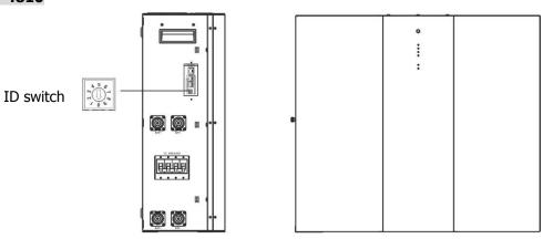
ID Switch indicates the unique ID code for each battery module. It's required to assign an identical ID to each battery module for normal operation. We can set up the ID code for each battery module by rotating the PIN number on the ID switch. From number 0 to 9, the number can be random; no particular order. Maximum 10 battery modules can be operated in parallel.
