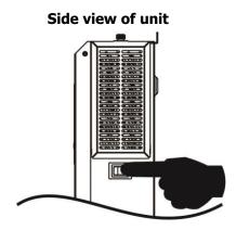
Once the unit has been properly installed and the batteries are connected well, simply press On/Off switch (located on the button of the case) to turn on the unit.
