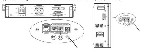
Step 2: Use supplied RJ45 cable (from battery module package) to connect inverter and Lithium battery.
