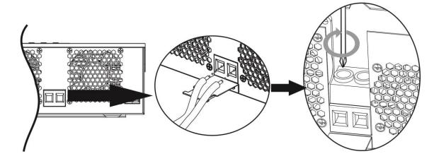
5. This step is only for RCT-AXVM2-PREM 1.2K-12V/RCT-AXVM2-PREM 2.5K-24V models. To firmly secure wire connection, you may fix the wires to strain relief with cable tie.
