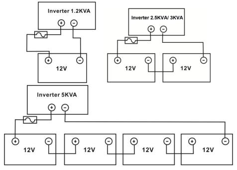
4. For RCT-AXVM2-PREM 1.2K-12V/RCT-AXVM2-PREM 2.5K-24V models, insert the battery wires flatly into battery connectors of inverter and make sure the bolts are tightened with torque of 2 Nm in clockwise direction. Make sure polarity at both the battery and the inverter/charge is correctly connected and conductors are tightly screwed into the battery terminals.
